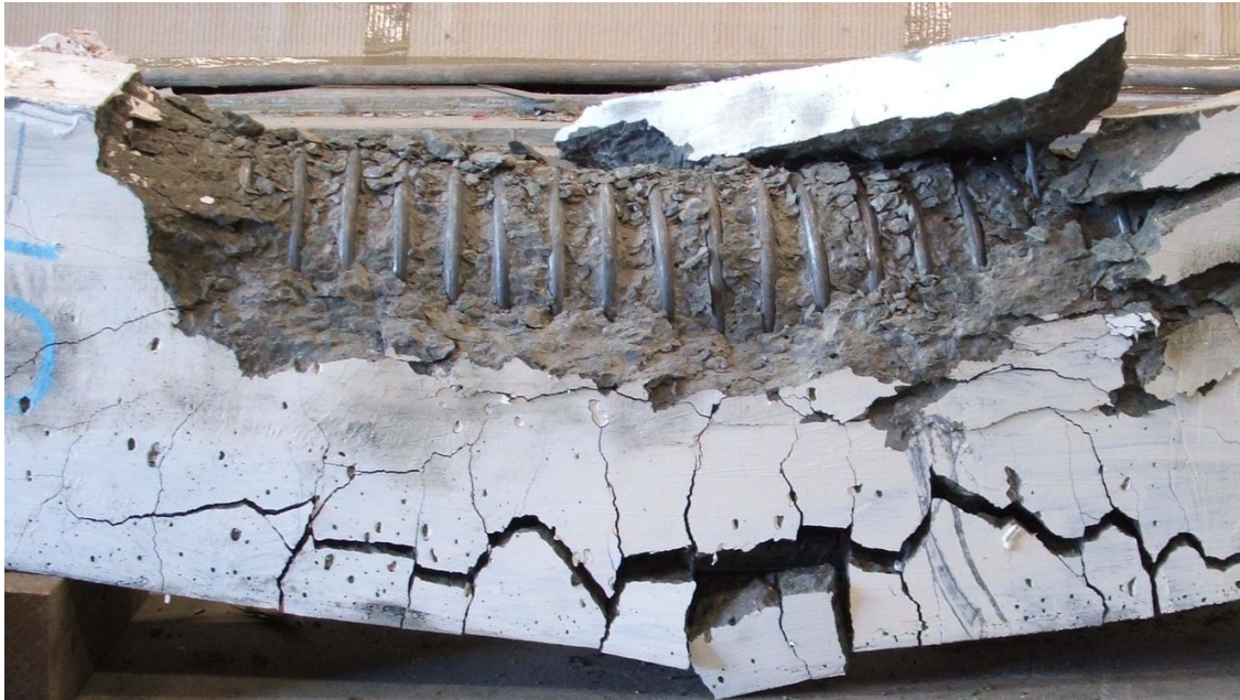
Figure 8. Crack patterns for Beam H-LR
