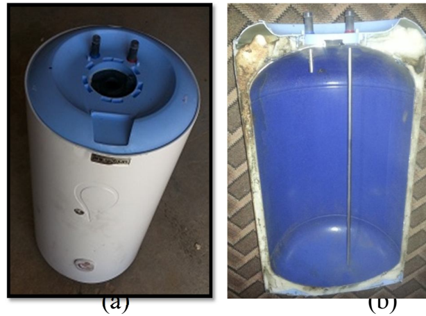
Figure 2. (a) Ordinary metallic boiler, (b) Vertical cross-section showing the inner part of metallic water boiler
