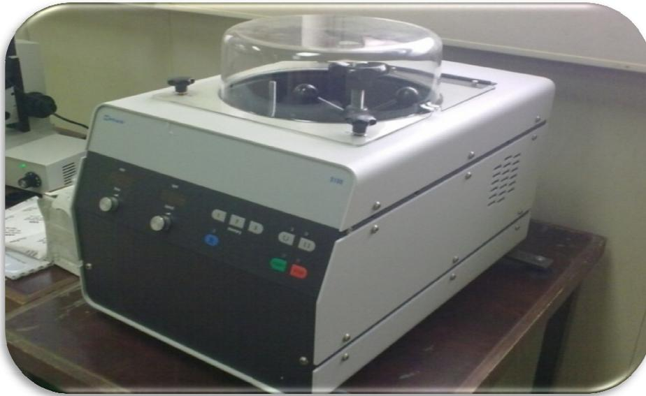
**Figure 1: The centrifugal ball mill used in the present work.**
