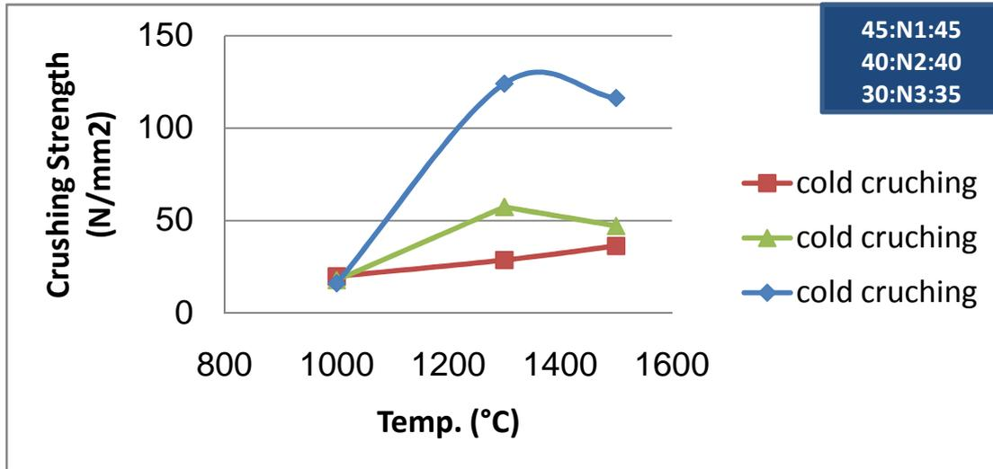
**Figure 5 : Cold crushing strength as a function of firing temperature**
