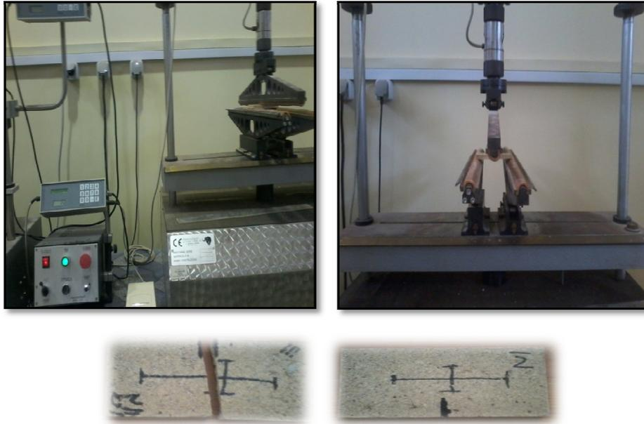
**Figure 2: Bending Tecno Tester and test samples.**
