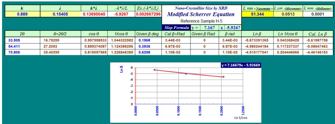
**Figure 3: An illustration of the computer calculation of the crystallite size for the powder milled for 5 hours**
