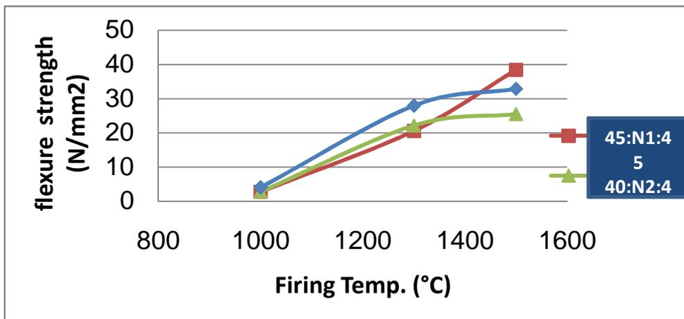
**Figure 6: Bending strength versus Firing temperature**
